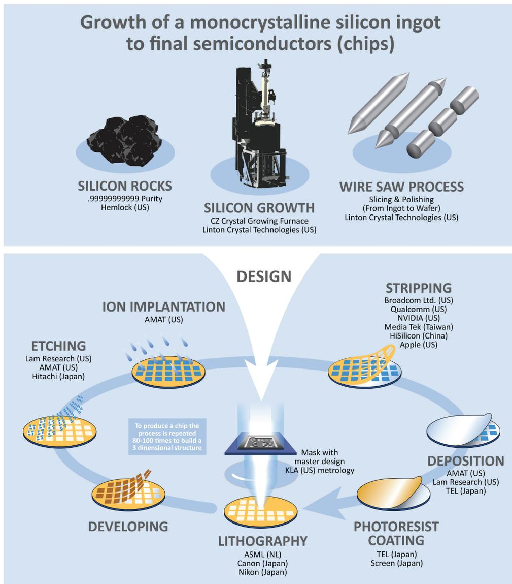
A single-wire saw cuts the top and bottom (crown and tail) off the ingot and then cuts it into sections of a manageable length (e.g. 500 mm). At this point, a multi wire saw will cut the sections into wafers. The final process steps in preparing the wafers for use in semiconductors are lapping, polishing, and washing. Layers of material are then applied to the prepared silicon wafer: a silicon oxide layer, a silicon nitride layer and a layer of a photoresist coating.
